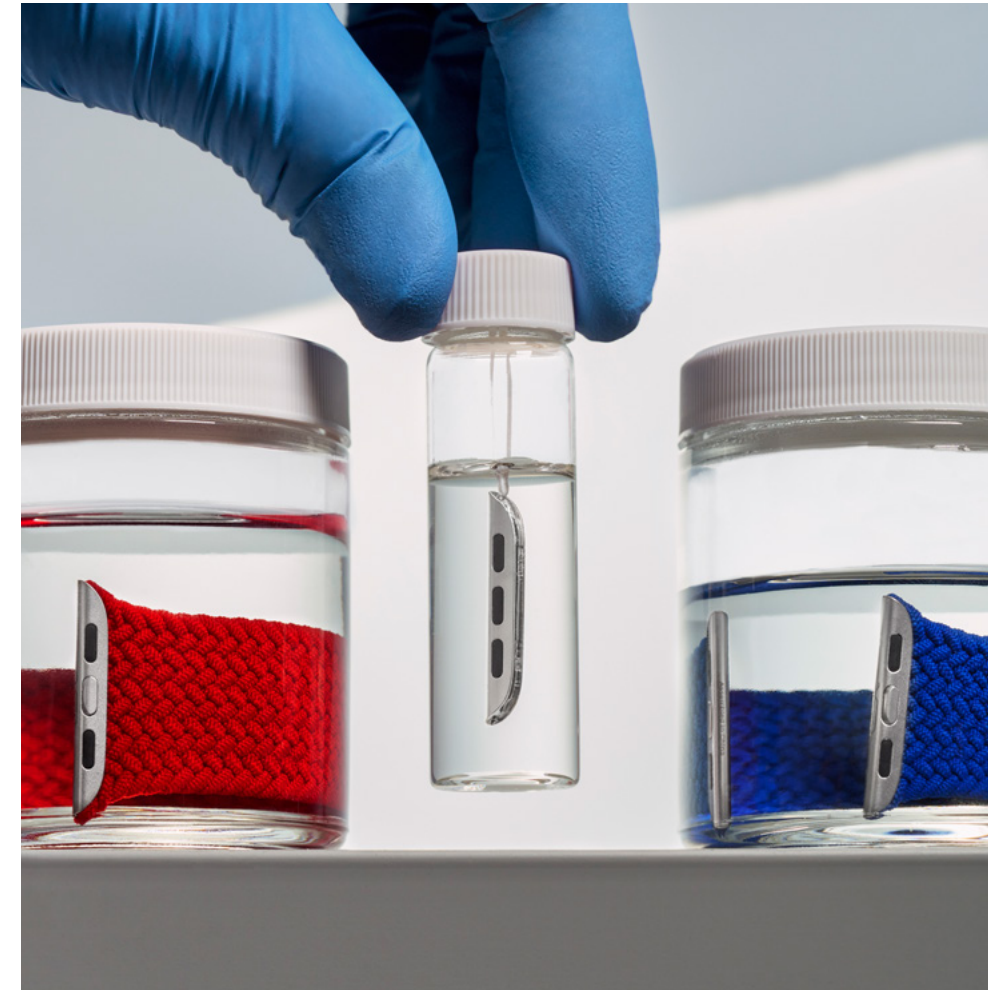
We test all our products, and place special attention on materials that come into prolonged skin contact. In this nickel leach test, we place Apple Watch straps in jars of artificial sweat to ensure the nickel, a potential allergen, stays where it belongs — in the product.
