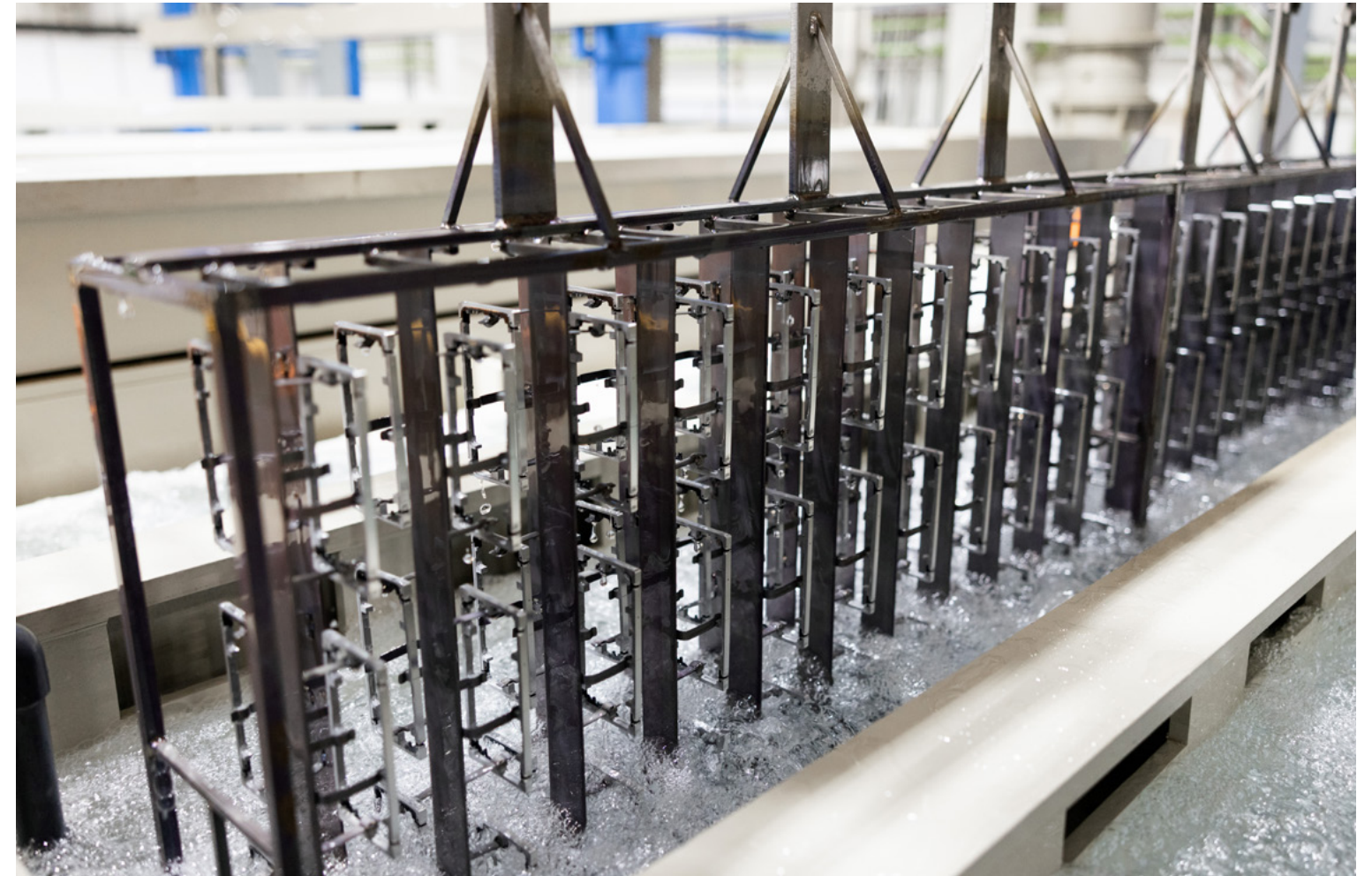
The aluminium anodising process is typically water-intensive. In 2019, we launched a pilot to seek to eliminate hazardous discharge and increase water efficiency from anodising. The cascade and counterflow rinsing processes, which helped retain 75 to 85 per cent of the water used during metal finishing, could save millions of gallons of freshwater annually when applied at scale.
